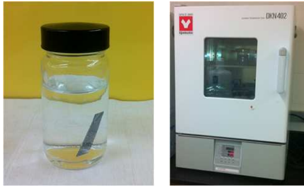
Figure 4: (Left) A silicon wafer is placed in a reaction vial containing the reaction solution, where the deposition side with ZnO faces down; (right) the reaction vial is placed in an convection oven.
