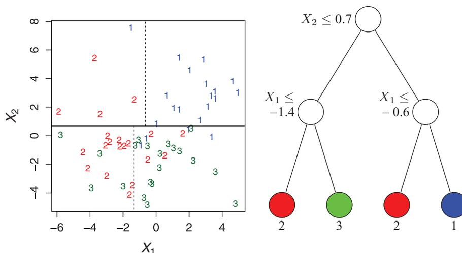
**FIGURE 1** | Partitions (left) and decision tree structure (right) for a classification tree model with three classes labeled 1, 2, and 3. At each intermediate node, a case goes to the left child node if and only if the condition is satisfied. The predicted class is given beneath each leaf node.
